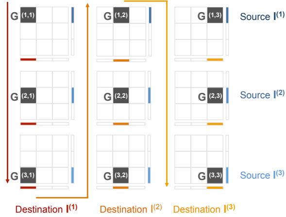
Fig. 2: M-Flash’s computation schedule for a graph with 3 intervals. Vertex intervals are represented by vertical (Source I) and horizontal (Destination I) vectors. Blocks are loaded into memory, and processed, in a vertical zigzag manner, indicated by the sequence of red, orange and yellow arrows. This enables the reuse of input (e.g., when going from G^{(3,1)} to G^{(3,2)} , M-Flash reuses source node interval I^{(3)} ), which reduces data transfer from disk to memory, boosting the speed.
